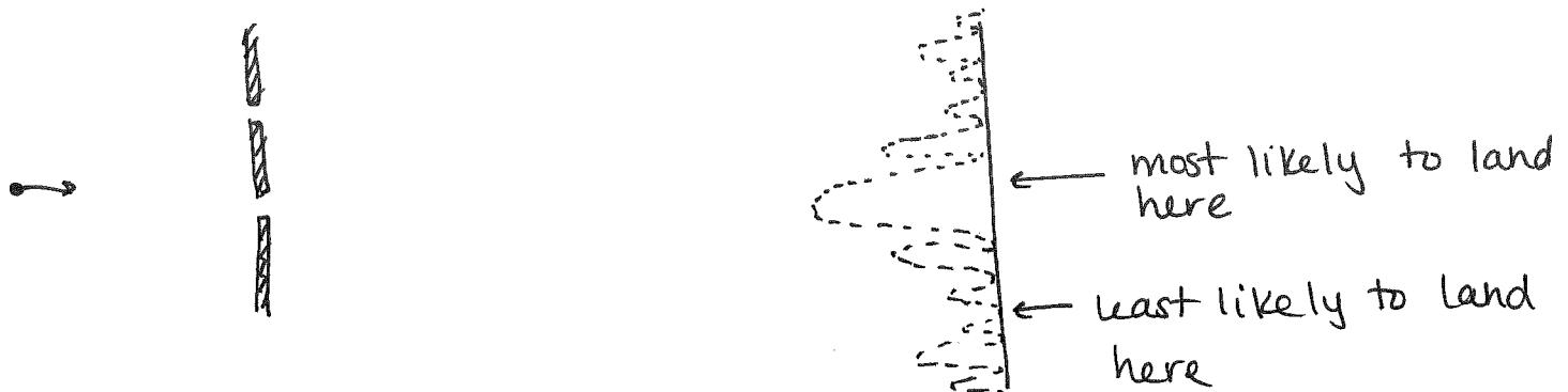
As we continue to send photons, we begin to "build up" the interference pattern, one photon at a time:
