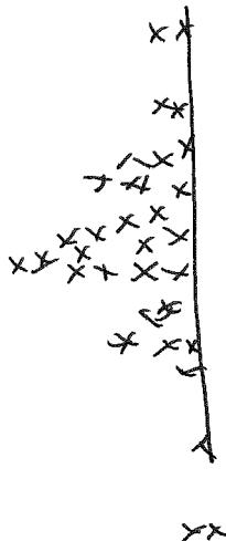
The "wave" that we see is the accumulation of many many individual particles. More importantly, the "wave" gives us the probability distribution (as a function of position on the screen) for a single photon.
